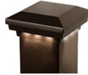
3in LED Post Cap Indirect Light 1.2 watts, 12 LEDS (3 LEDS per side), 156 Lumens, with an approximate effective Lumen output of 39 Lumens, 4,000 Kelvin P/N: LE045311 M B=Black, W=White, Z=Bronze
